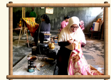
Fine work using the canting, a pen-like tool to apply liquid hot wax.
