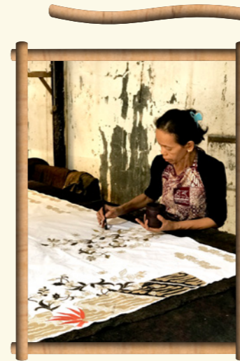
Dyeing using the brush technique, or colet .
